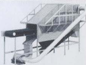
Weight screening equipmet (Wind selector)
